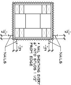
\* NAIL LATH EVERY 6" DOWN EACH CORNER 1 1/2" FROM EDGE WITH FASTENER PENETRATING MIN. OF 1" INTO STUD.
